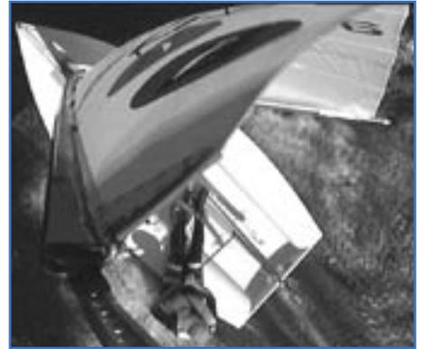
WB-Sails uses digital video camera attached to the top of the mast to record sail shape on the water.
